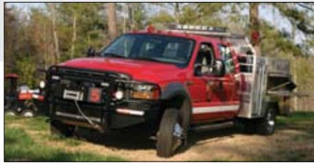
Brush trucks are capable of reaching remote areas and areas not easily accessible by fire engines and trucks. They are highly effective vehicles that are smaller and more maneuverable, allowing them to negotiate narrow pathways, off-road trails and golf cart paths. They are equipped with foam capabilities that, in wildland fires, suppress better than water.
