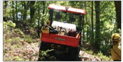
The smaller, highly maneuverable Kubota assists brush trucks in fighting wildland fires. The Kubota's firefighting capabilities can be replaced with a medical response skid unit, enabling it to perform emergency medical transport in off-road environments.
