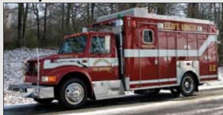
This unit is used for technical rescue response, heavy extrication and industrial rescues and is equipped with a light mast for nighttime operations.
