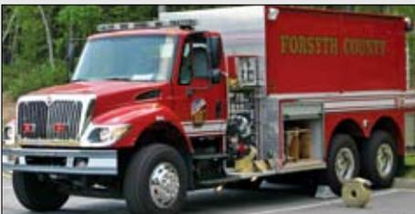
Tankers are used to transport water to scenes that do not have positive water supplies.
